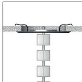
Mounting on plasterboard-ceiling
